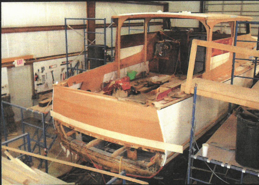
Left: The transom was in perilous condition and had to be completely rebuilt. Top Right: A laminated replacement frame is “spliced” onto one found to be rotten. About 30 frames, or ribs, were repaired in this fashion. Bottom Right: Decades of paint are stripped away to get down to Movie Pilar ’s bare mahogany.
