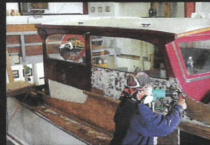
Left: The transom was in perilous condition and had to be completely rebuilt. Top Right: A laminated replacement frame is “spliced” onto one found to be rotten. About 30 frames, or ribs, were repaired in this fashion. Bottom Right: Decades of paint are stripped away to get down to Movie Pilar ’s bare mahogany.
